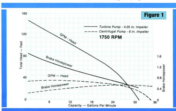
PD pump – power directly proportional to head (rather than capacity), with maximum power required at shutoff (where it's the lowest for a centrifugal pump) and a steep head-capacity curve – the RTP is a kinetic pump (Figure 1).
