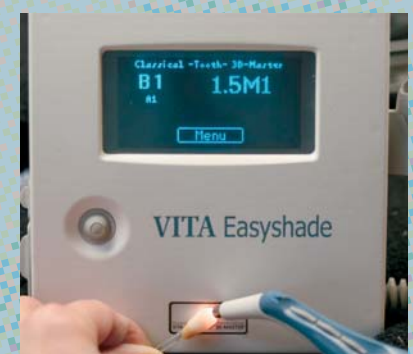
FIGURE 4. The Easyshade system (Vident, Brea, CA) provides an immediate digital reading of the cervical, body, and incisal shades using either the Vitapan Classical and/or Vitapan 3-D Master shade guides.
