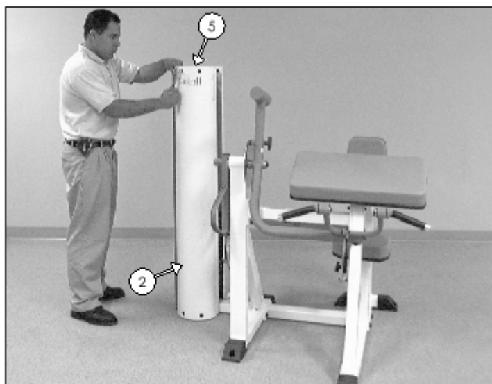
FIG. 25 Affix the Weight Shroud (#2) to the bottom of the Weight Stack Frame (#1) and at the top of the Guide Rod Retainer (#5) using four Hex Head Cap Screws 1/4-20 X 3/4 (#61), and four Flat Washers 1/4" (#52).
