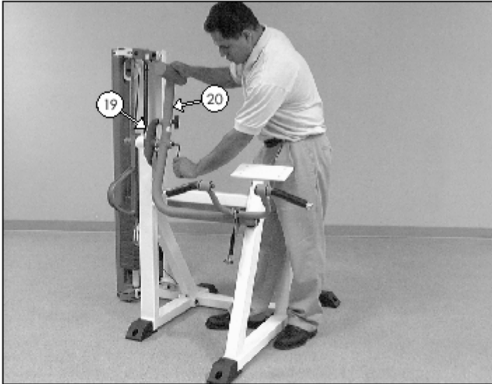
FIG. 19 Attach the Swing Arm (#20) to the axle of the Circular Plate (#19) and secure it into place using one Button Head Socket Cap Screw 3/8-16 X 1 (#35), one Split Lock Washer 3/8" (#96), and one Chrome Washer 3/8 X 1 1/2 (#36).
