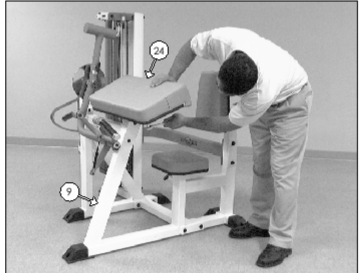
FIG. 24 Attach the Arm Curl Pad (#24) to the Main Frame (#9) using two Hex Head Cap Screws 3/8-16 X 1 1/4 (#63), and two Flat Washers SAE 3/8" (#53).
