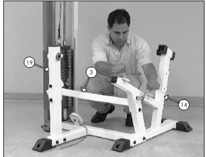
FIG. 14 Attach the Arm Support (#3) to the Upright Support (#19) using two Hex Head Cap Screws 1/2-13 X 4 1/2 (#54), four Flat Washers SAE 1/2" (#47), and two Nylon Insert Lock Nuts 1/2-13 (#66). Next, attach the Arm Support (#3) to the Seat Frame (#14) using two Hex Head Cap Screws 1/2-13 X 3 1/2 (#53), four Flat Washers SAE 1/2" (#47), and two Nylon Insert Lock Nuts 1/2-13 (#66).
