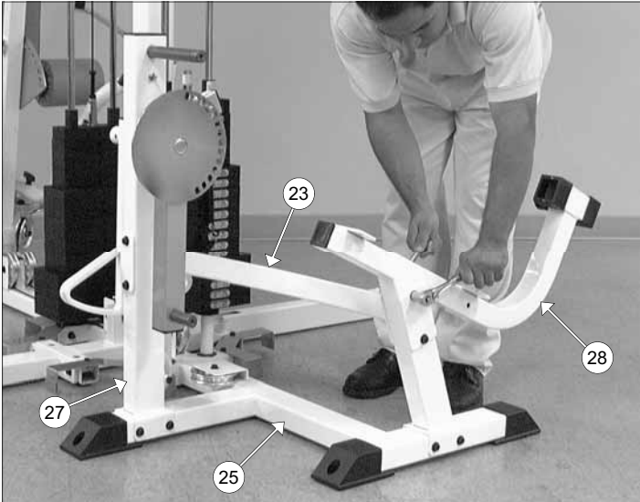
FIG. 55 Next, attach the Leg Extension Arm Support (#23) to the Leg Extension Front Frame (#27) using two Hex Head Cap Screws 3/8-16 X 4 1/4 (#104), four Flat Washers SAE 3/8" (#93), and two Nylon Insert Lock Nuts 3/8-16 (#119). Next, attach the other end of the Leg Extension Arm Support (#23) to the Leg Extension Seat Frame (#28) using two Hex Head Cap Screws 3/8-16 X 3 1/4 (#101), four Flat Washers SAE 3/8" (#93), and two Nylon Insert Lock Nuts 3/8-16 (#119).
