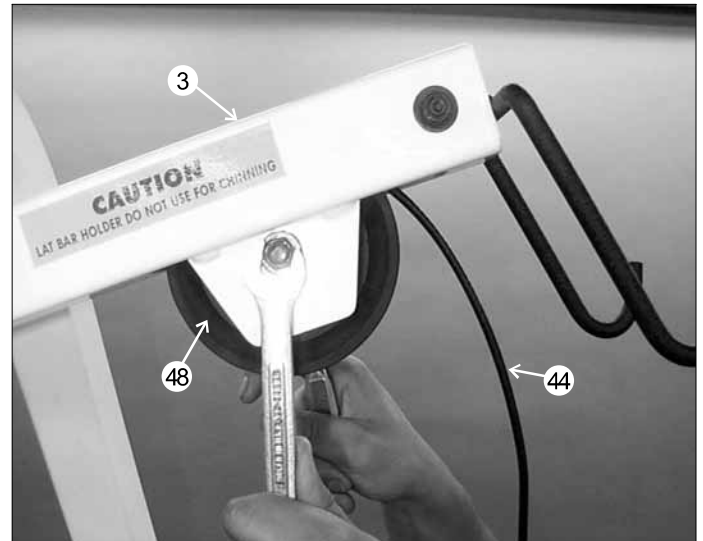
FIG. 32 Raise the Lat Cable (#44) into place, as shown above, with the Lat Cable (#44) fitted into the groove of the Nylon Pulley 4 1/2 Rd. (#48). Secure into place using one Hex Head Cap Screw 3/8-16 X 1 3/4 (#57), two Flat Washers SAE (#73) and one Nylon Insert Jam Lock Nut 3/8-16 (#69). Route the Lat Cable (#44) over the Nylon Pulley 4 1/2 Rd. (#48) and into the tube of the Top Pulley Assembly (#3) . Use Fig. I on page 15 and Fig. B on page 16 for further detailed illustration cable routing.
