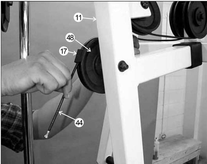
FIG. 37 Now install a Nylon Pulley 4 1/2 Rd. (#48) and one Cable Retainer Bracket (#17) onto the Front Upright (#11) , as shown, and secure it using one Hex Head Cap Screw 3/8-16 X 3 3/4 (#52), two Flat Washers SAE 3/8 (#73) and one Nylon Insert Jam Lock Nut 3/8-16 (#69). Route the Lat Cable (#44) over the pulley as shown. Use Fig. I on page 15 and Fig. B on page 16 for further detailed illustration cable routing. Note: Be sure the Cable Retainer Bracket (#17) is positioned as shown above.
