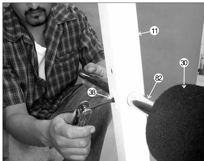
FIG. 26 Now, insert a Foot Roll Tube 1 X 25 (#82) through the Front Upright (#11) , as shown above. Secure the Foot Roll Tube 1 X 25 (#82) using a Set Screw 3/8-16 X 1/2 (#38). Use the Hex-Key 3/16 (#80) tool for securing the Set Screw 3/8-16 X 1/2 (#38). Next, insert two Foam Foot Rolls 7 X 4 X 1 (#30) and two Plastic Insert Caps 1" Rd. (#75) into the the Foot Roll Tube 1 X 25 (#82) .
