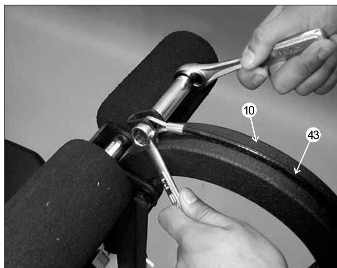
FIG. 44 Attach the Leg Ext Cable (#43) to the Leg Ext Arm (#10) , as shown above. Secure using one Hex Head Cap Screw 3/8-16 X 1 (#59), two Flat Washers SAE 3/8 (#73) and one Nylon Insert Jam Lock Nut 3/8-16 (#69). Refer to Fig. F on page 16 for further clarification of this assembly.
