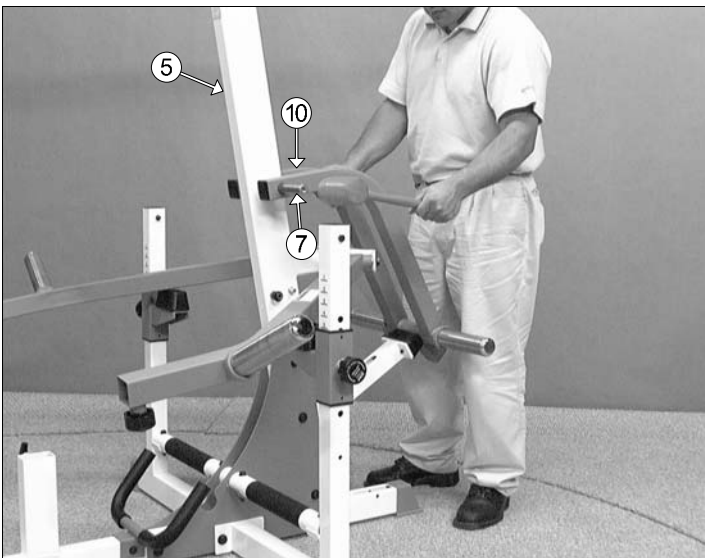
FIG. 18 Attach the Weight Carriage (#10) to the Main Frame (#5) , in the position as shown above. Next, using a rubber mallet, insert the Pivot Axle 1 X 8 1/8 (#7) through the holes of the Weight Carriage (#10) and the receptacle of the Main Frame (#5) until it is flush with both sides of the Weight Carriage (#10) .
