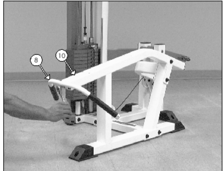
FIG. 22 Attach the Handles (#8) to the Main Frame (#10) using two Hex Head Cap Screws 3/8-16 X 1 1/4 (#54) and two Split Lock Washers 3/8" (#80).
