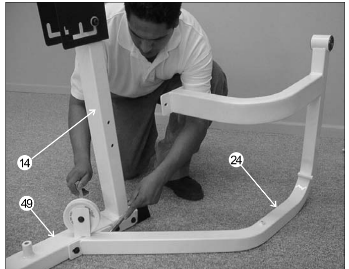
FIG. 6 Attach the Leg Extension Main Frame (#24) , as shown above, to the Platform (#49) and secure it into place using two Hex Head Cap Screws 3/8-16 X 3 3/4 (#108), four Flat Washers SAE 3/8 (#12) and two Nylon Insert Jam Lock Nuts 3/8-16 (#74). Note: Do not completely fasten the hardware at this time, as it will be completely secured later in the assembly process.
