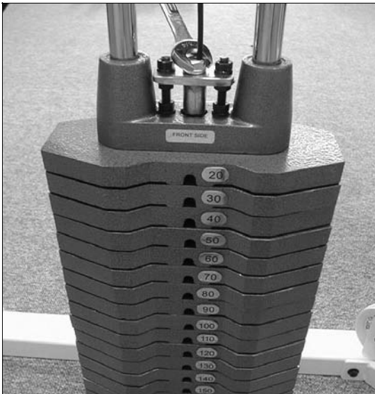
FIG. 45 Next, attach the Lat Cable (#86-labeled with tape A) to the Top Plate/Selector Bar (#42) and secure it into place using one Split Bolt 1/2-13 X 1 (#101) and one Split Washer 1/2" (#102) , as shown above. Refer to Fig. 73 on page 21 for further detailed illustration of this assembly. Note: Be sure this hardware assembly is securely fastened.
