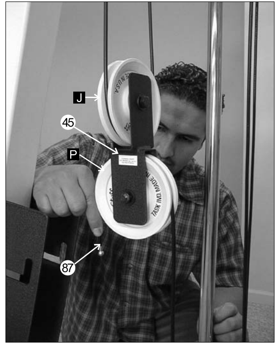
FIG. 54 Next, route the Low Row Cable (#87-labeled with tape B) over the Nylon Pulley 4 1/2 Rd. (#17-Labeled P) located on the Offset Pulley Bracket (#45) , as shown above. Refer to the Cable Mapping Diagram on page 20 for further detailed illustration of this routing.
