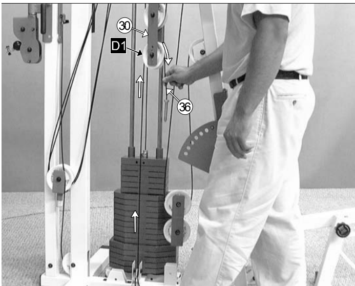
FIG. 62 Route the Tension Cable (#36) up to the Closed-End Adjustable Pulley Bracket (#30) and over the Nylon Pulley 4 1/2 Rd (#67-Labeled D1) , as shown above.
