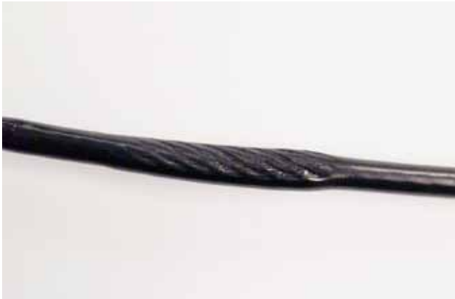
"NECKING", STRECHED CABLE COVERING
