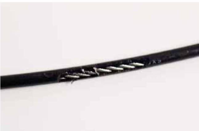
A TEAR IN THE CABLE COVER
