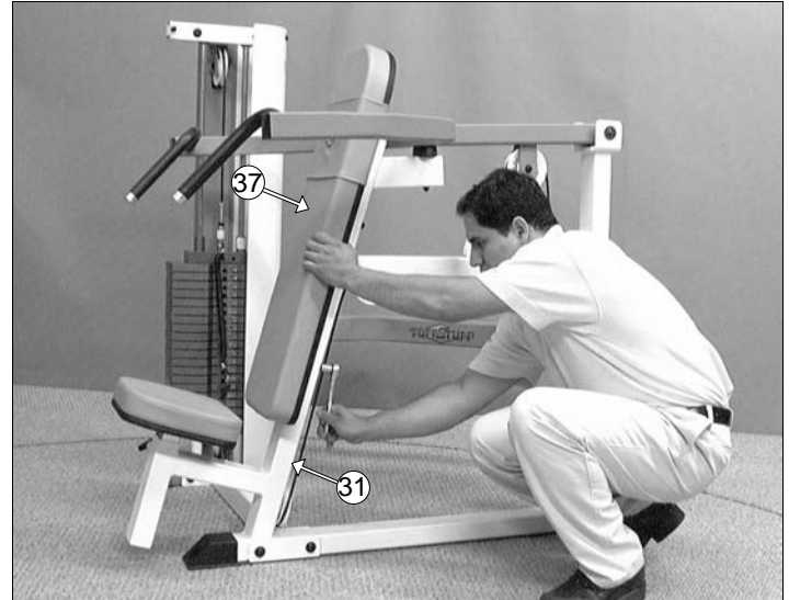
FIG. 20 Affix the Back Pad (#37) to the Shoulder Press Main Frame (#31) , in the position as shown above, using four Hex Head Cap Screws 3/8-16 X 3 (#52), and four Flat Washers SAE 3/8" (#19).
