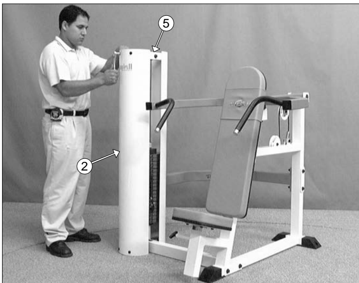
FIG. 21 Affix the Weight Shroud (#2) to the bottom of the Weight Stack Frame (#1) and at the top of the Guide Rod Retainer (#5) using four Hex Head Cap Screws 1/4-20 X 3/4 (#21), and four Flat Washers 1/4" (#20).
