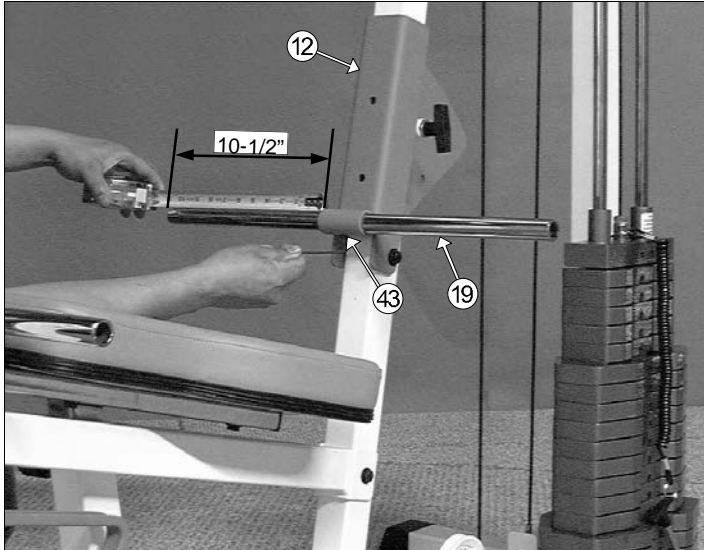
FIG. 54 Secure the Foot Roll Tube 1 X 23-3/4 (#19) to the Adjustable Back Pad Bracket (#12) using a Set Screw 1/4-20 X 1/4 (#43) . Use the supplied Hex Key 1/8" (#86) for securing the Set Screw 1/4-20 X 1/4 (#43) into the threaded socket located on the Adjustable Back Pad Bracket (#12) .
