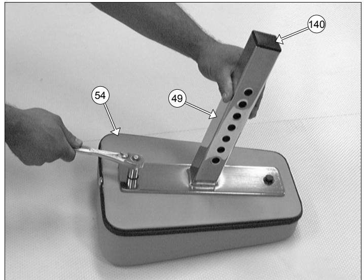
FIG. 16 Using a rubber mallet, insert one Plastic Insert Cap 1 3/4" Sq. (#140) into the tube-end of the Adjustable Back Pad Tube (#49) . Next, attach the Adjustable Back Pad Tube (#49) to the Back Pad (#54) using two Hex Head Cap Screws 3/8-16 X 1 1/4 (#99), and two Flat Washers SAE 3/8" (#94).
