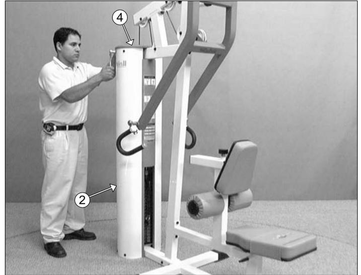
**FIG. 38** Affix the **Weight Shroud (#2)** to the bottom of the **Weight Stack Frame (#1)** and at the top of the **Guide Rod Retainer (#4)** using four Hex Head Cap Screws 1/4-20 X 3/4 (#17), and four Flat Washers 1/4" (#16).
