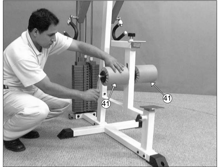
**FIG. 30** Attach two **Foam Rolls 1 X 5 1/2 X 7 1/4 (#41)** to the **Foot Roll Tube (#35)** and secure them into place using two Hex Head Cap Screws 3/8-16 X 1 1/2 (#66).
