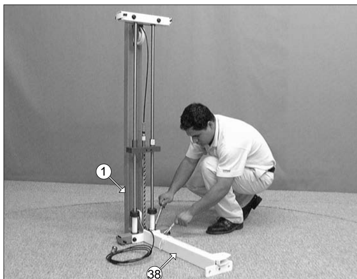
FIG. 1 On a flat surface, attach the Bottom Cross Brace (#38) to the assembled Weight Stack Frame (#1) , in the position as shown above, and secure it into place using two Hex Head Cap Screws 1/2-13 X 3 1/2 (#24), four Flat Washers SAE 1/2" (#29), and two Nylon Insert Lock Nuts 1/2-13 (#22).
