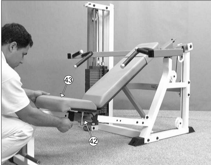
FIG. 23 Affix the Seat Pad (#43) to the Bench Slide Carriage (#42) , in the position as shown above, using four Hex Head Cap Screws 3/8-16 X 1 1/4 (#75) , and four Flat Washers SAE 3/8" (#19) .
