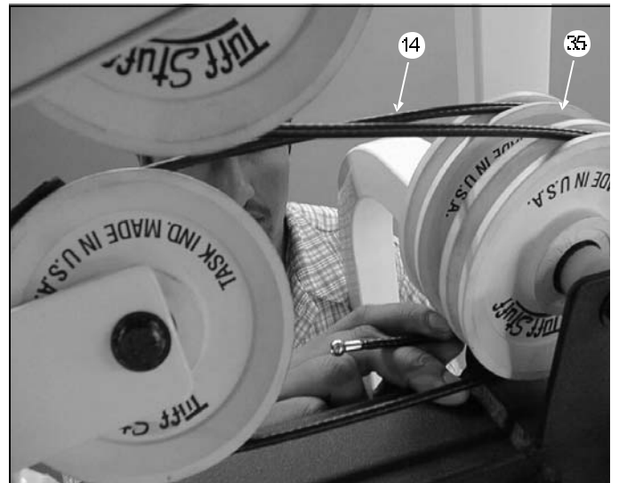
FIG. 44 Continue to route the Lat Cable (#14) over the Nylon Pulley 4 1/2 Rd. (#35), then under, as shown above. Refer to Fig. 1 on page 17 and Fig. B on page 18 for further detailed illustration of this cable routing.
