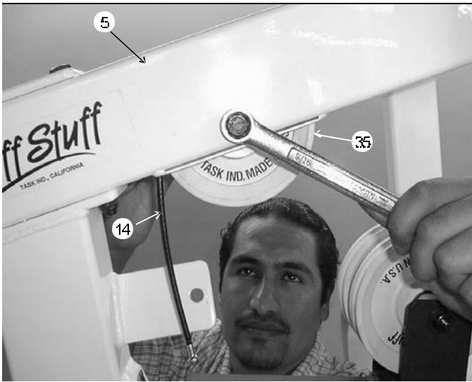
FIG. 41 Insert the Lat Cable (#14) and one Nylon Pulley 4 1/2 Rd (#35) into the Top Pulley Assembly (#5) and secure it using one Hex Head Cap Screw 3/8-16 X 2 1/2 (#78), two Flat Washers SAE 3/8 (#90) and one Nylon Insert Jam Lock Nut 3/8-16 (#86). Refer to Fig. 1 on page 17 and Fig. B on page 18 for further detailed illustration of this cable routing.
