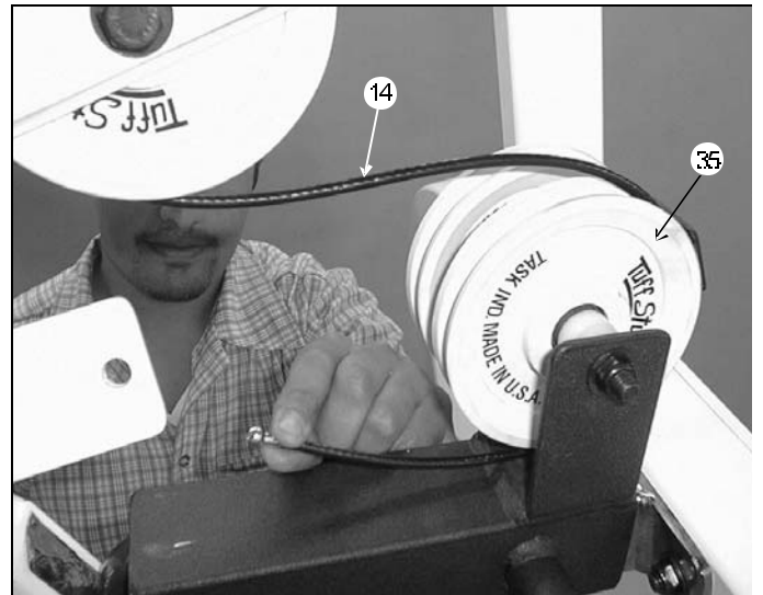
FIG. 42 Route the Lat Cable (#14) over, then under the Nylon Pulley 4 1/2 Rd. (#35), as illustrated above. Refer to Fig. 1 on page 17 and Fig. B on page 18 for further detailed illustration of this cable routing.
