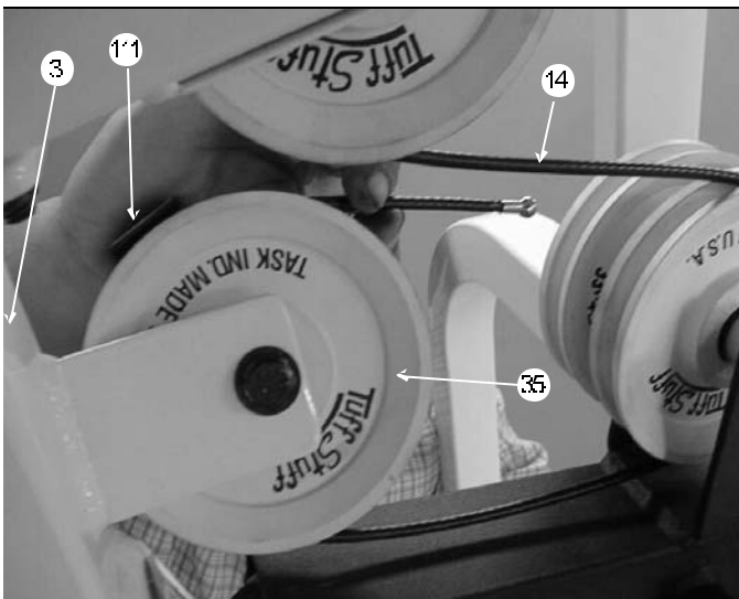
FIG. 43 Next, attach a Nylon Pulley 4 1/2 Rd. (#35) to the pulley bracket on the Front Upright (#3) and secure it using one Hex Head Cap Screw 3/8-16 X 1 3/4 (#79), two Flat Washers SAE 3/8 (#90), one Nylon Insert Jam Lock Nut 3/8-16 (#86) and one Cable Retainer Bracket (#111) . Next, route the Lat Cable (#14) under, then over the Nylon Pulley 4 1/2 Rd. (#35), as shown above. Refer to Fig. 1 on page 17 and Fig. B on page 18 for further detailed illustration of this cable routing.
