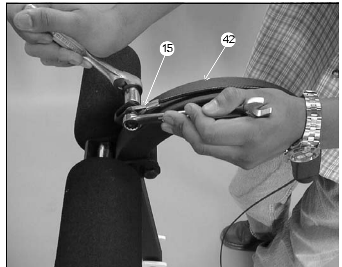
FIG. 52 Attach the Leg Extension Cable (#15) to the Leg Extension Arm (#42) and secure it using one Hex Head Cap Screw 3/8-16 X 1 (#81) and one Nylon Insert Jam Lock Nut 3/8-16 (#86). Refer to Fig. F on page 18 for further detailed illustration of this cable routing.
