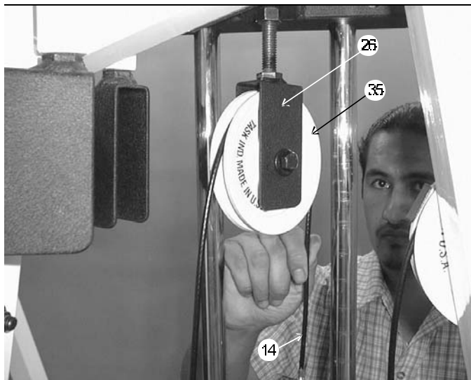
FIG. 47 Insert a Nylon Pulley 4 1/2 Rd. (#35) into the Adjustable Pulley Bracket (#26) and secure it using one Hex Head Cap Screw 3/8-16 X 1 3/4 (#79), two Flat Washers SAE 3/8 (#90) and one Nylon Insert Jam Lock Nut 3/8-16 (#86). Route the Lat Cable (#14) through the Adjustable Pulley Bracket (#26) , as shown above.
